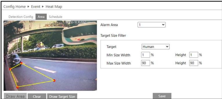
Click the “Draw Area” button and then click around the area where you want to set as the alarm area in the image on the left side (the alarm area should be a closed area). Click the “Clear” button to delete the alarm area. Click the “Save” button to save the settings.
