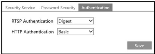
The screenshot shows a web interface with three tabs: "Security Service", "Password Security", and "Authentication". The "Authentication" tab is active. It contains two dropdown menus: "RTSP Authentication" set to "Digest" and "HTTP Authentication" set to "Basic". A "Save" button is located at the bottom right of the form.
