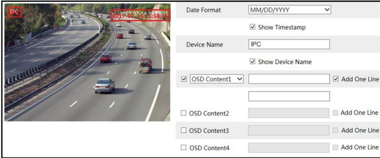
Set time stamp, device name, OSD content and picture overlap here. After enabling the corresponding display and entering the content, drag them to change their position. Then click the “Save” button to save the settings.
