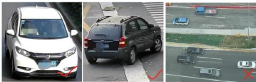
5. Make sure cameras can view objects for at least 2 seconds in the detected area for accurate detection.
