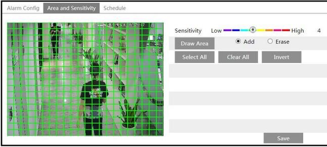
Move the “Sensitivity” scroll bar to set the sensitivity. Higher sensitivity value means that motion will be triggered more easily.
